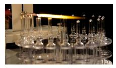
The Ampulmatic Ampule Sealer is a dramatic step up in ease, speed and consistency of ampule sealing. It automatically spins the ampules while melting the top with an oxygen/propane flame to form a positive hemispherical seal. When combined with the optional Purge Gas Injector and/or the optional Liquid Filler, the Ampulmatic-10 represents a start-to-finish solution,
